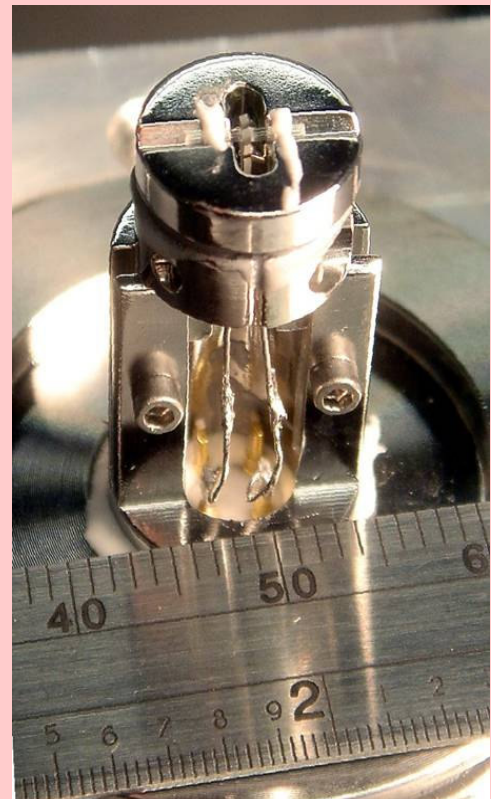
Quartz resonator photoacoustic sensing cell
