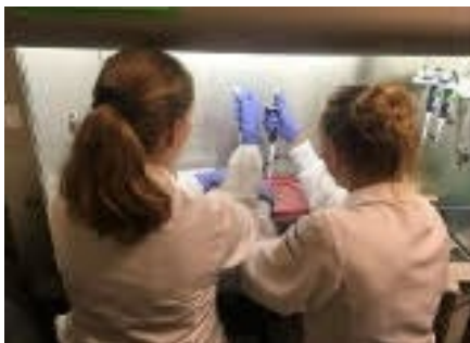
Dr. Verena Charwat (left) and Dr. Berenice Charrez (right) perfusing cardiac microtissues with preservation solution prior to supercooling. (Photo credit: M. J. Powell-Palm)
