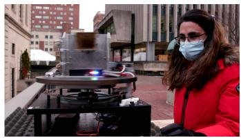
Columbia Engineering students take millimeter wave channel measurements for the COSMOS advanced wireless research testbed in West Harlem. COSMOS is a cloud-enhanced open software defined mobile wireless testbed for city-scale deployment. (Credit: Columbia Engineering)
